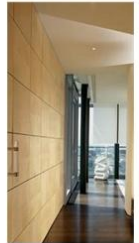
4. Storage. Additional storage to be within wall spaces around kitchen hallways. To be constructed from Spray finish MDF with concealed push click openings,
